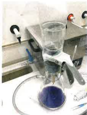
Figure 6. Filtration unit with air suction
