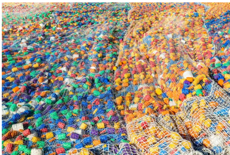
Figure 32. Hydro Sound Dampers (HSD) net with rubber or plastic bubbles (Photo: Vattenfall).
