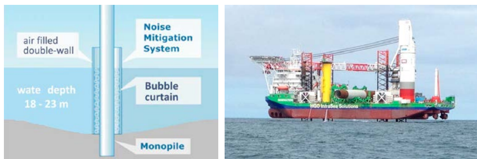
Figure 31. Left: An illustration of the IHC-NMS system with an air-filled double wall that encircles the pile and an internal bubble curtain, from Koschinski and Ludemann (2013). Right: IHC-NMS system in use (the red-white casing) during pile driving for a wind farm in the German North Sea (Photo: Markus Linné, FOI).
